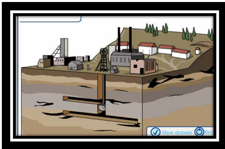
A deep level mine with a shaft
